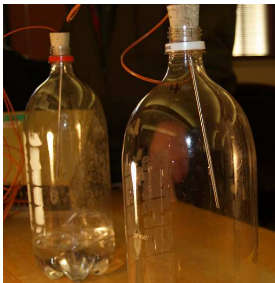
FIGURE 2. Thermocouple in a two-liter bottle. Note that the thermocouples are not perfectly vertical, nor are they likely to be perfectly centered. The near thermocouple points away from the lamp and residue from the label shields the thermocouple.
