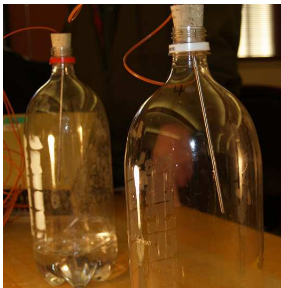
FIGURE 2. Thermocouple in a two-liter bottle. Note that the thermocouples are not perfectly vertical, nor are they likely to be perfectly centered. The near thermocouple points away from the lamp and residue from the label shields the thermocouple.
