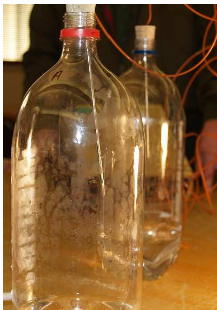
FIGURE 3. A thermocouple in a two-liter bottle. Note that this thermocouple points toward the lamp, and has a reflector from the residue of the label torn from the bottle.
