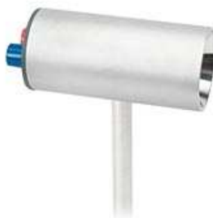
FIGURE 4. A Moll-type thermopile. Picture from Cenco on-line catalog.
