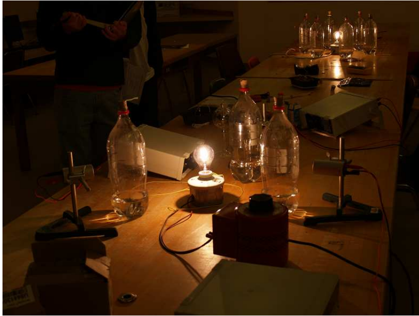
FIGURE 1. Two separate set-ups running at the same time. While it looks like our lab is bathed in mood-lighting this is an illusion. The extremely bright filaments fooled my automatic camera. The room was brightly lit. The nearest set-up uses Moll-type thermopiles, while the distant setup is more like the NOAA description, except with thermocouples replacing lab thermometers.
